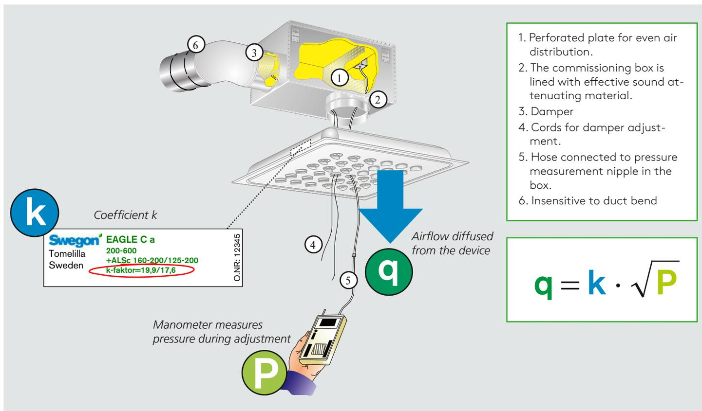
A well balanced air distribution system is quiet, free of draught, energy efficient and it distributes air evenly between the rooms. Therefore it is important that the system is accurately commissioned.
