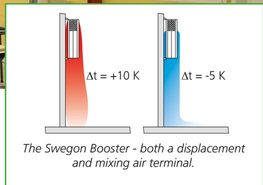
Thanks to the Varizon® air distribution system, the diffusion pattern of the chilled air can also be adjusted to prevent draughts.
